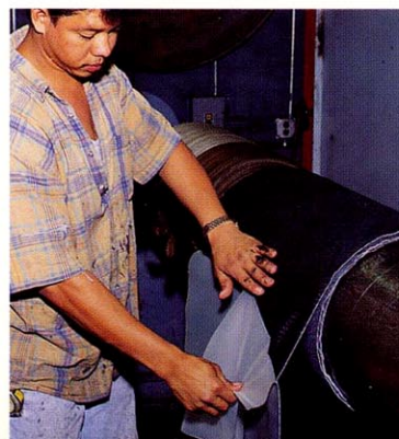
8 Building eccentric reducers becomes more difficult because the mandrel rotates off center. This varies the working distance between the product and the assembler, and requires exceptional coordination.
