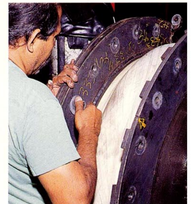
10 When the nylon body wrap is finished, the steel mold plates that form the rubber flanges are bolted in place to retain the flanges during the curing process.
