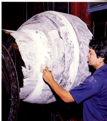
8 Building eccentric reducers becomes more difficult because the mandrel rotates off center. This varies the working distance between the product and the assembler, and requires exceptional coordination.
