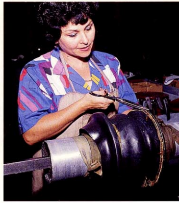
3 Before the steel flange forms can be bolted or clamped in position, the perimeter is carefully trimmed.
