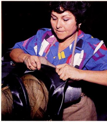
2 When the expansion joint nears completion, the exterior sheath is pulled up to form the cover on the back of the flange.
