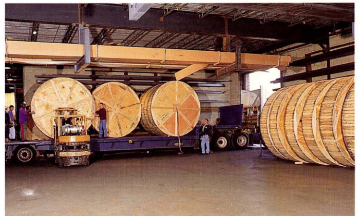
7 Hydro testing is another phase and all products undergo one final quality control evaluation before shipment. Once approved, large expansion joints are packed securely in wood spool crates for added protection on their journey.
