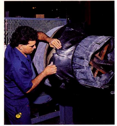
4 Products are formed on a mandrel. Its shape fits the inside contour of the product. Concentric reducers are built with the small and large diameters on opposite ends, joined by a cone shape transition section.
