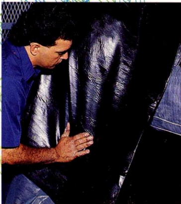
7 Cover application is the final stage of reducer body building.
