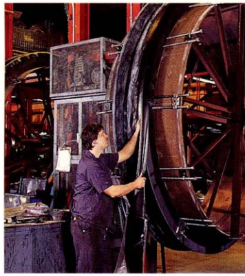
1 Although every assembly follows similar procedures, the complexity of each job varies with its shape, size and pressure requirements. Shown here are 96 inch diameter joints under construction.
