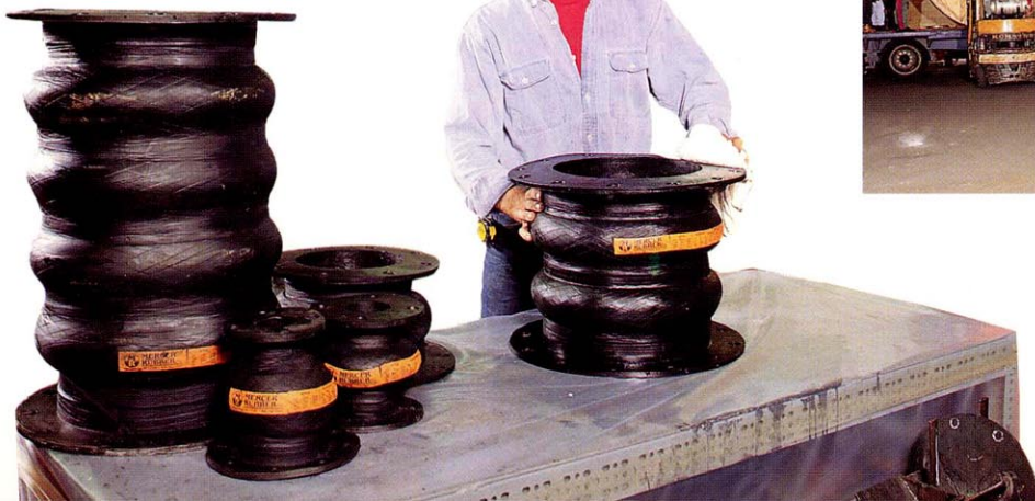
6 During final inspection, all rubber parts are trimmed, cleaned and painted. Finally, ductile iron or steel backup rings are attached to the flanges and checked for hole alignment.
