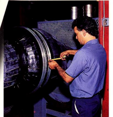
6 To prevent swelling, large diameter expansion joints are generally reinforced with high-tensile wire or steel hoops. This process requires precise application of both wire and uncured rubber fillers.
