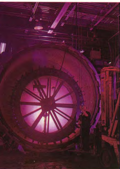
Custom built autoclaves make steam curing oversize expansion joints commonplace.
